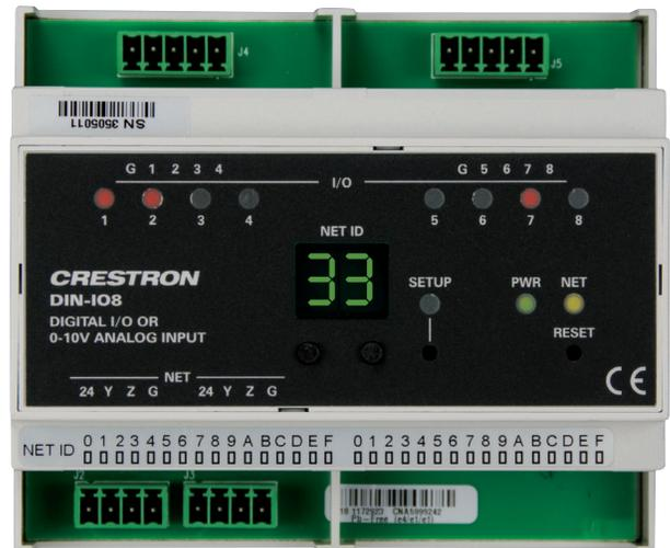
NET: (2) 4-pin 3.5mm detachable terminal blocks, paralleled; Cresnet slave port
