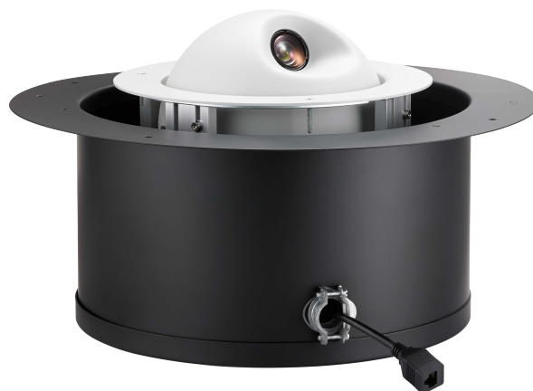
The RoboFLIP 30 HDBT features one HDBaseT output
