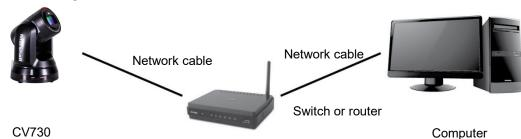
2. To connect directly through network cable, the IP address of the computer should be changed so that it is on the same network segment as the camera e.g.: The factory-preset default IP address of CV730 is 192.168.100.100. The computer IP address must be set with the same network segment, such as 192.168.100.101, so that the computer can be connected correctly with the camera
